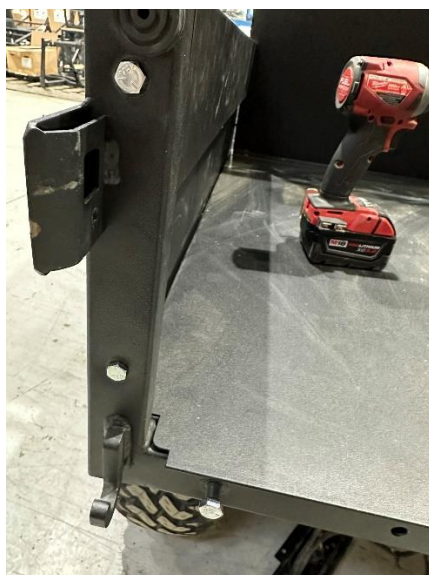
Figure 9: 1/4" bolts installed through the rear support into the side panels.
