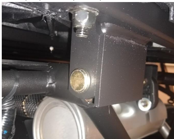
Figure 3: Bed hinge pin fully inserted through the bed hinge bracket and bed stub tube.
