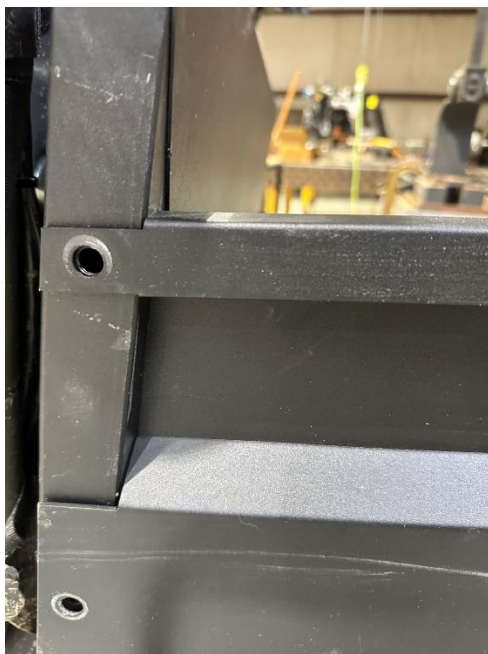
Figure 6: This shows the side panel properly aligned with the header of the bed.
