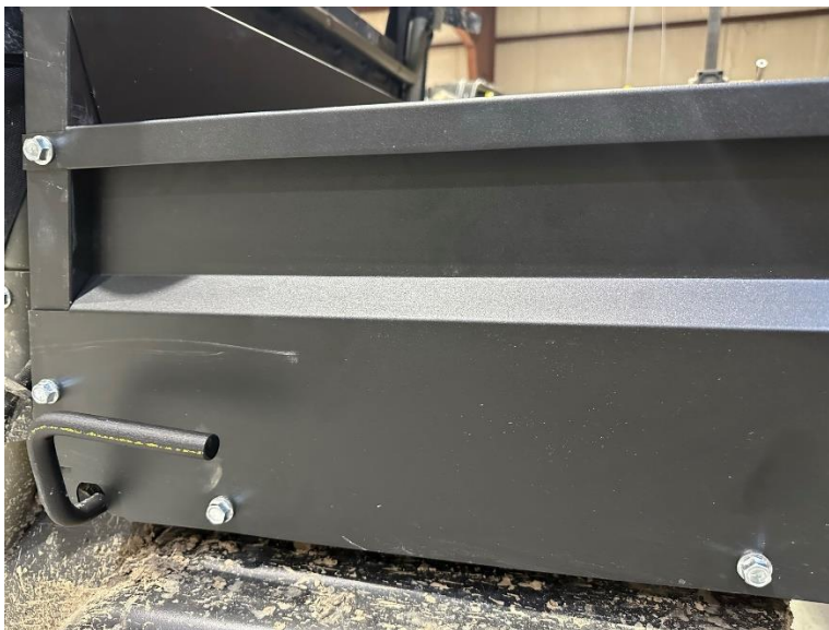
Figure 7: Four of the five side bolts shown completely installed.
