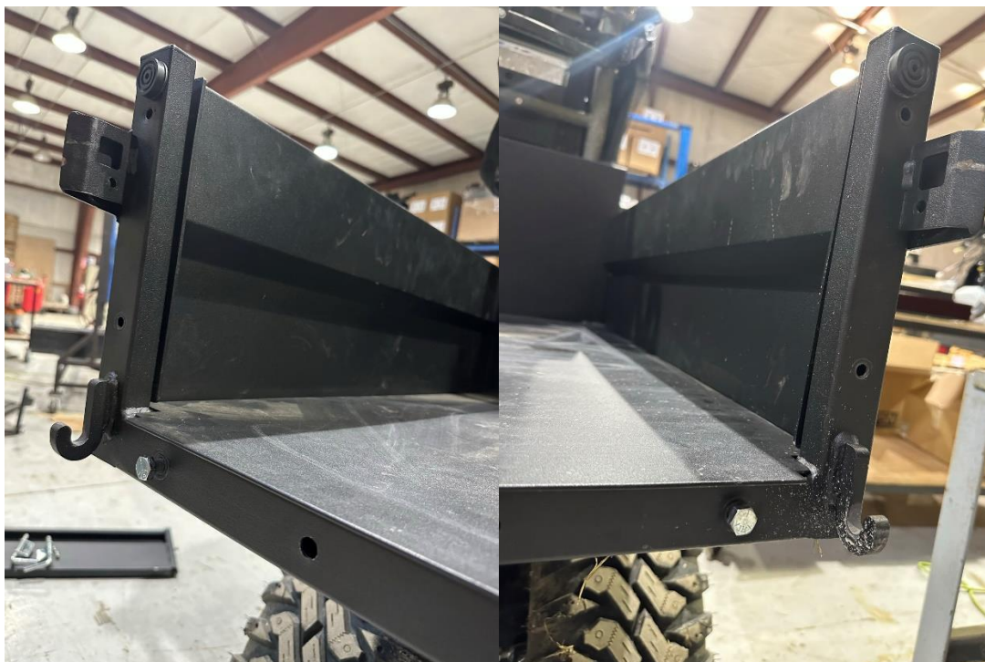
Figure 8: The left and the right side of the rear support weldment lined with the side panels.
