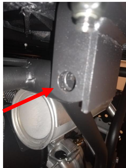
Figure 2: Bed hinge bracket lined up with the bed stub tube.
