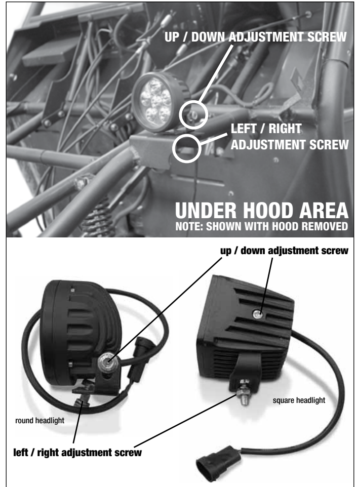
figure 4.18 (headlight adjustment screw locations)
