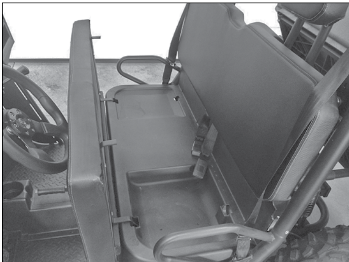
figure 4.1 (seat removal - pull forward and lift up)
