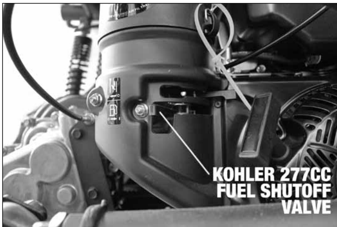
figure 4.20 (engine fuel shutoff valve located on 277cc Kohler)
