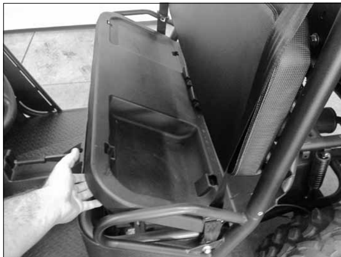
figure 4.2 (underseat storage tray removal - lift up and pull out.)
