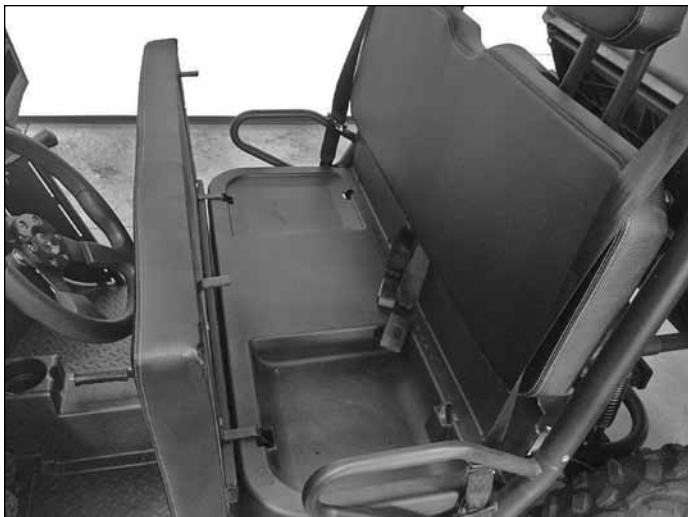
figure 4.1 (seat removal - pull forward and lift up)
