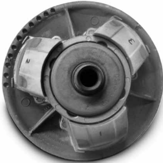
tab positoning on sliding flange
