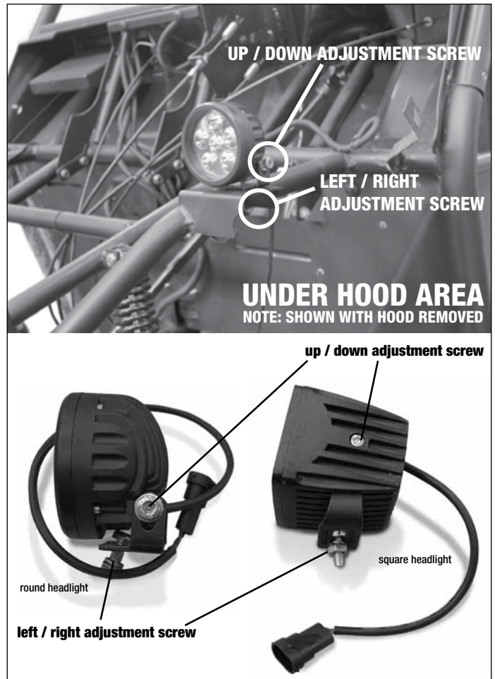
figure 4.19 (headlight adjustment screw locations)
