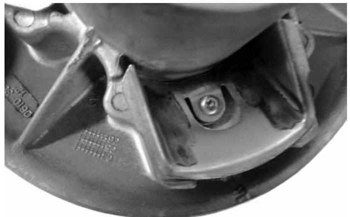
the sliding flange ramps once cleaned
