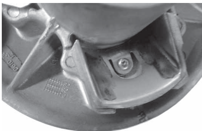
the sliding flange ramps once cleaned
