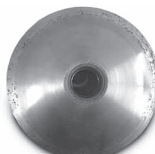
sliding flange after cleaning
