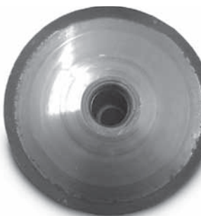
sliding flange before cleaning
