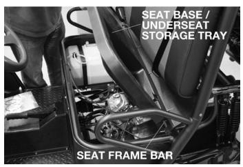
Place front tabs of seat bottom into the slots on the underseat storage tray and lower seat into position.
