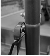
Place the cage on front vehicle frame tubes and seat back. Insert a 5/16" x 2" socket head bolt through all four joints. The head of the bolt should be on the outside of the vehicle. Put a curved washer on the threaded end of the bolt. Place a 5/16" nylock nut on the bolts.
