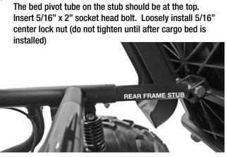
Place the cargo bed on the vehicle and insert a 5/8" x 4" hex head bolt through each pivot bracket and frame stub tube. The bolt heads should be facing the center of the vehicle with the nuts facing the outside.
