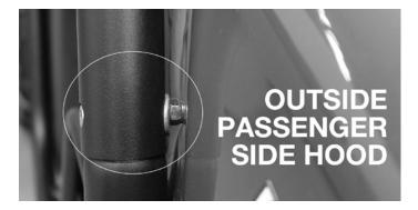
Tighten the nylock against the bent washer VERY tightly to secure the Brushguard.
