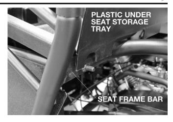
Secure underseat storage tray by pushing down firmly around the plastic seat bottom wrap.
