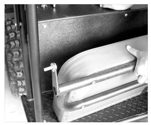
This subsequent photo shows the final installation into the side weldment, with the Nylock nut on the outside of the assembly.
