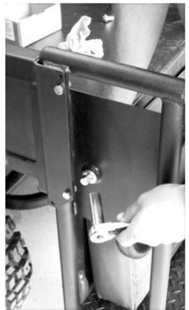
The photo below shows the final installation of the seat bottom.
