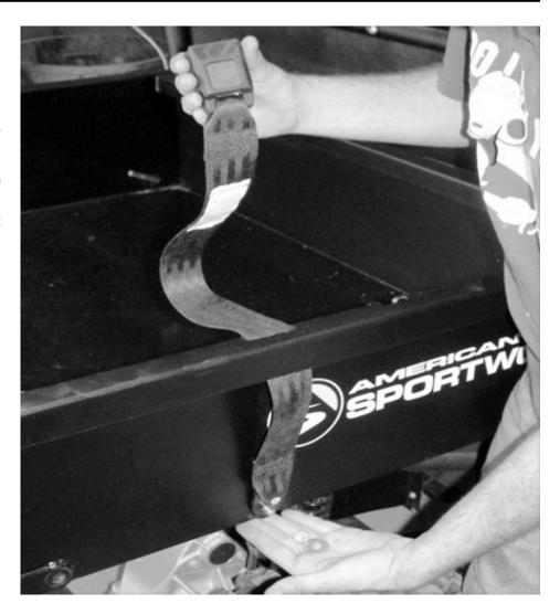
Step 7: Installation of the seat belt latch.
