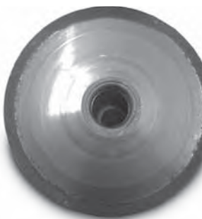
sliding flange before cleaning
