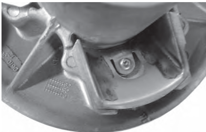
the sliding flange ramps once cleaned
