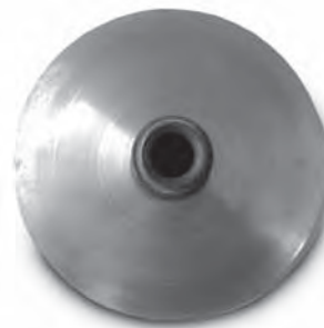
fixed flange after cleaning
