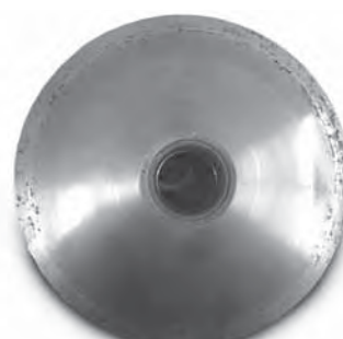
sliding flange after cleaning
