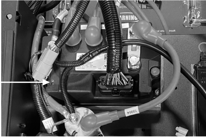
Motor Controller with Blink Code Light
