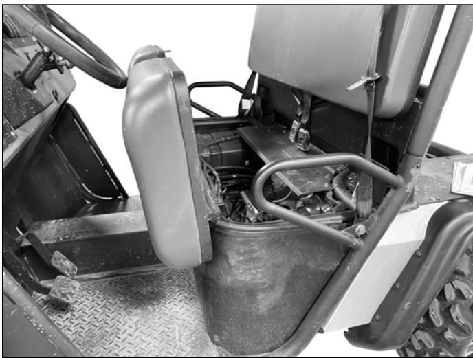
figure 4.1 (seat removal - lift rear and tilt forward)
