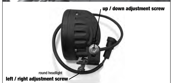
figure 4.16 (headlight adjustment screw locations)
