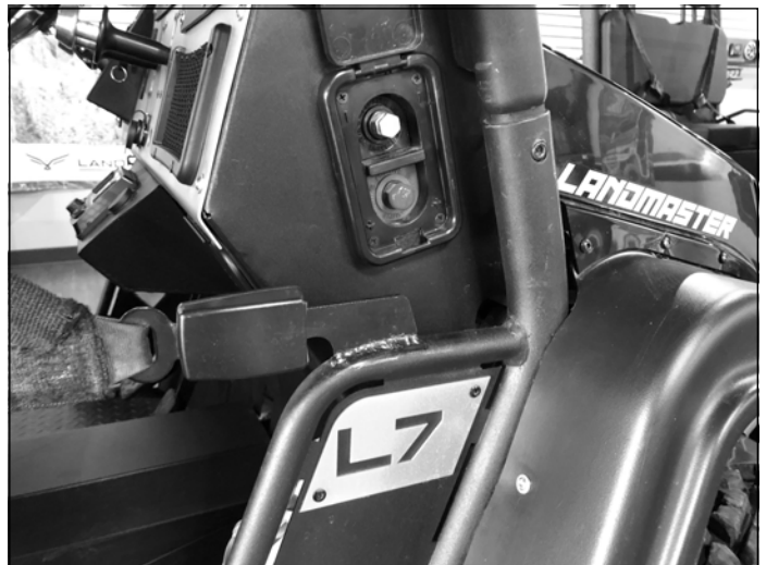
figure 4.20 (battery charging port)
