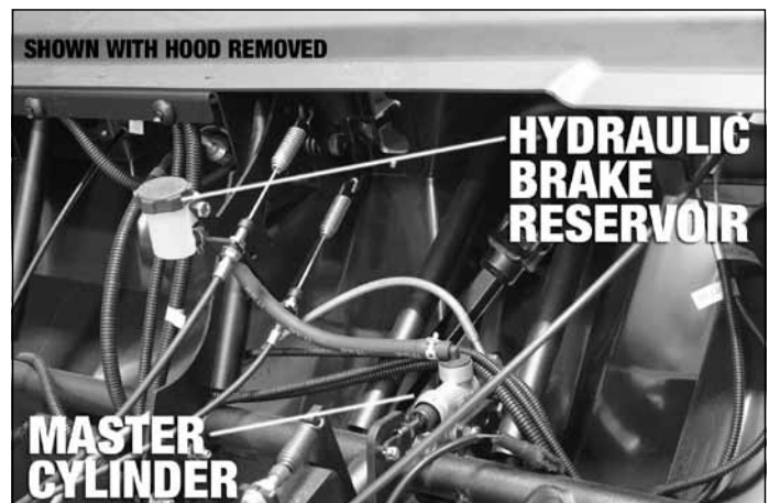
figure 4.17 (hydraulic brake reservoir location)
