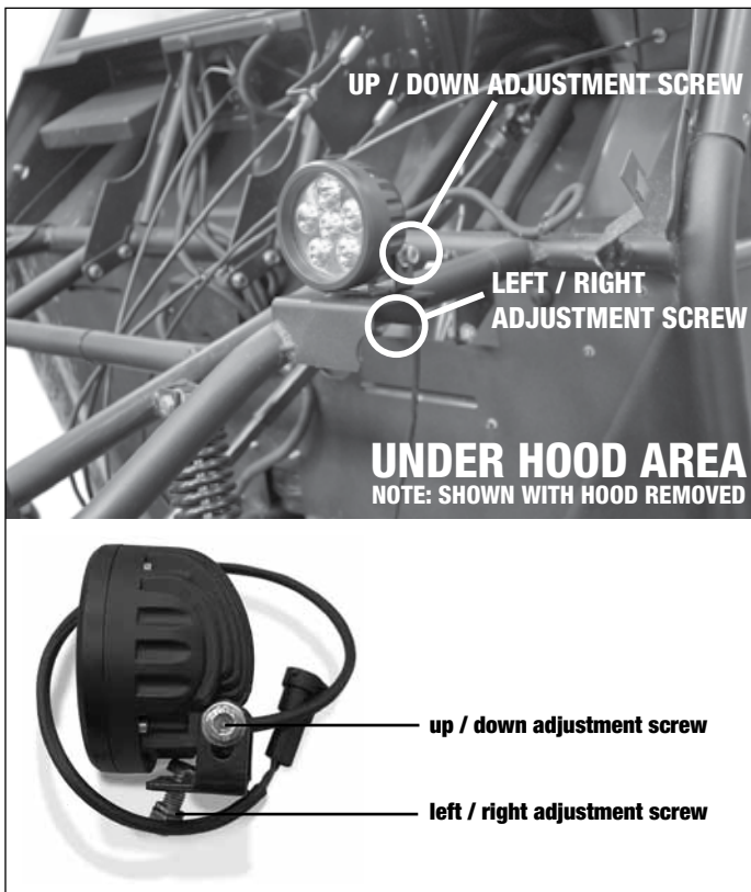
figure 4.18 (headlight adjustment screw locations)
