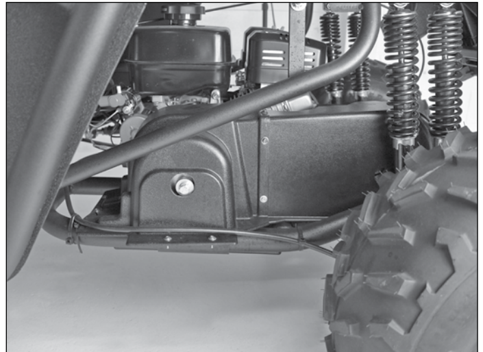
figure 4.5 (drive belt cover - 2WD unit shown)
