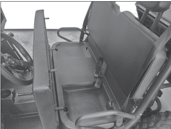
figure 4.1 (seat removal - pull forward and lift up)
