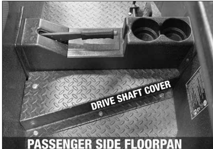
figure 4.11 (4WD drive shaft location)
