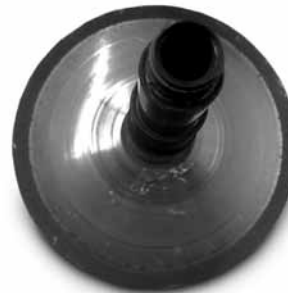
fixed flange before cleaning
