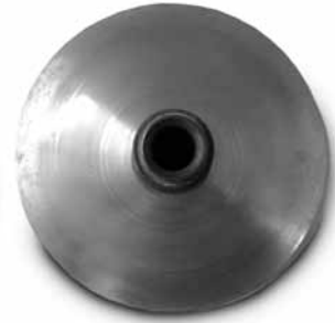
fixed flange after cleaning
