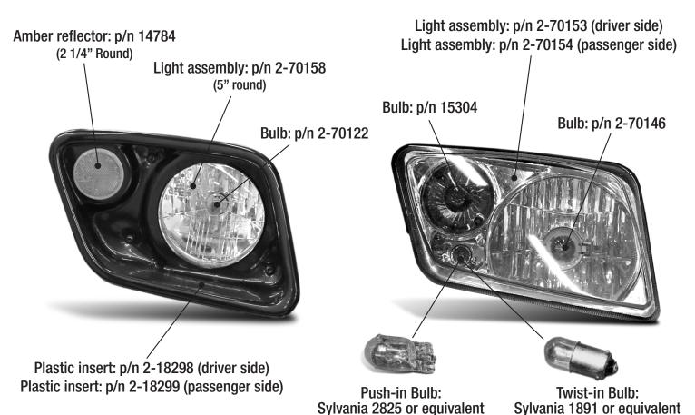
Depending on your year of manufacture, this housing either has a "push-in" or "twist-in" bulb
