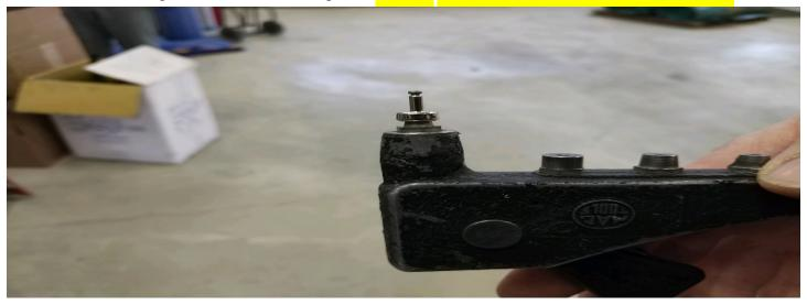
5.BEFORE rivet is installed into frame, put a little dab of silicone then snap into frame. The silicone will help prevent any rust from forming
