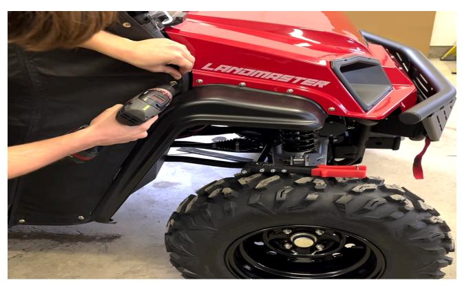
3. Use a 1/8" drill bit, hold snap to frame (pull tightly to assure tight fit and finish) and drill through snap on enclosure, partially into frame PAGE 3 (SECOND PICTURE)
