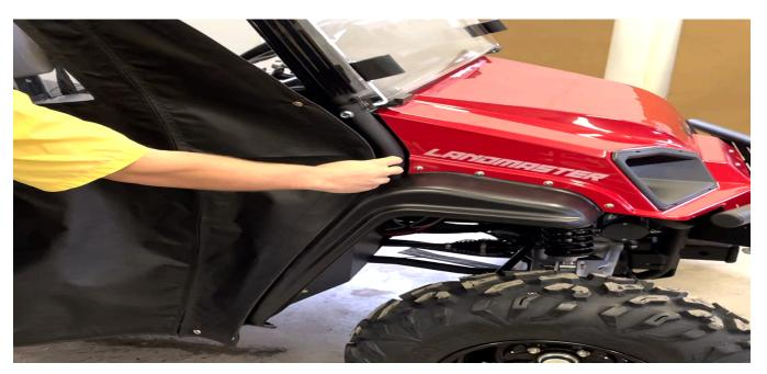
2. Line up first snap as shown on page 3. (TOP PICTURE). Snap should line up with bolts on fender underneath LANDMASTER sticker
