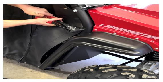
After first rivet is installed, move to opposite end of enclosure, and install second rivet. Alternate back and forth, making sure enclosure fits tightly, but NOT TOO TIGHTLY
