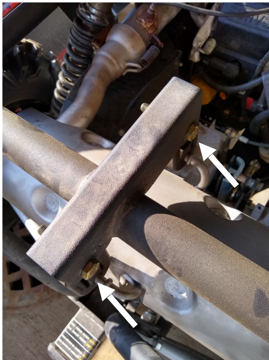
Figure 1.4: This figure shows the bolts to remove to release the muffler.
