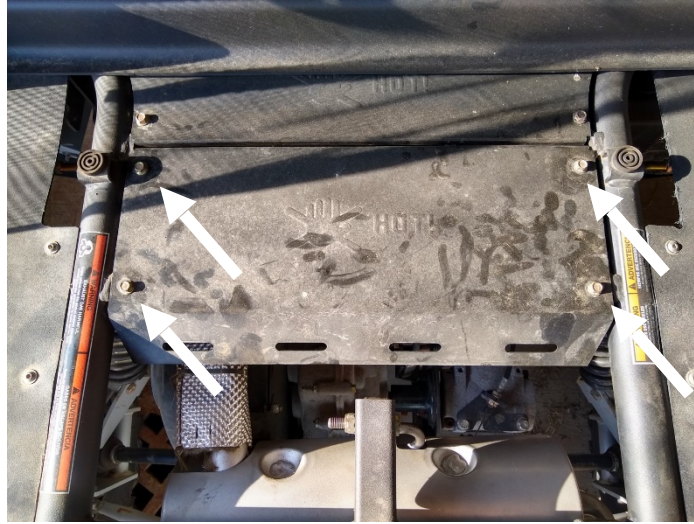
Figure 1.1: This figure shows the locations for the rear heat shield bolts.
