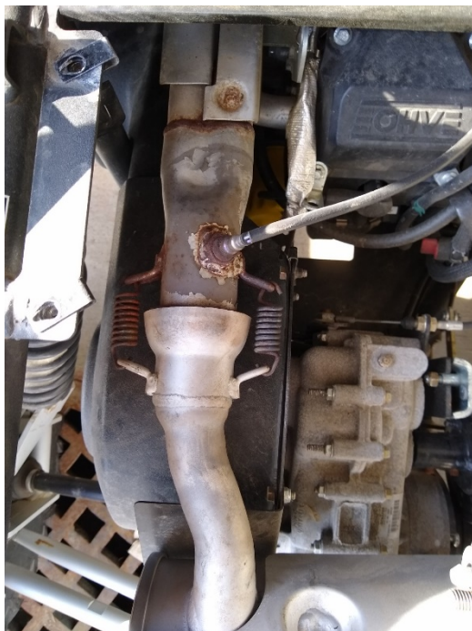
Figure 1.3: This figure shows the heat wrap removed from the exhaust pipes.
