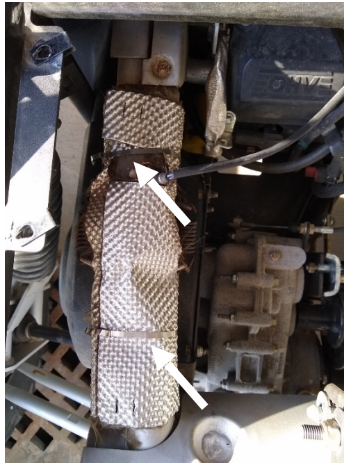
Figure 1.2: This figure shows the straps to cut for the heat wrap removal.
