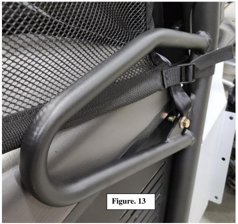
13. All straps should be checked and made taught before use. This net is to be used anytime the vehicle is in motion. Failure to use this product as intended can put users at risk of serious injury or death. The net is to be in the upright stored position or removed when not in use.
