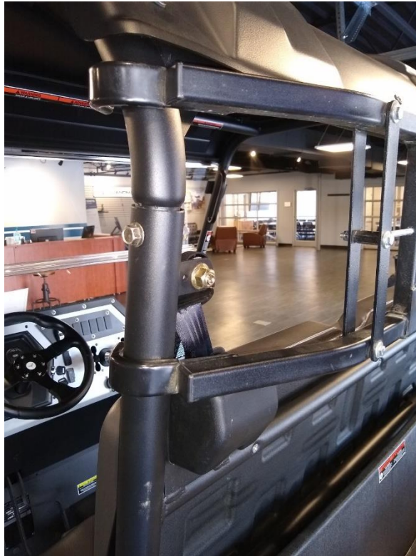
Figure 3: Recommended gun rack location on b-pillar.
