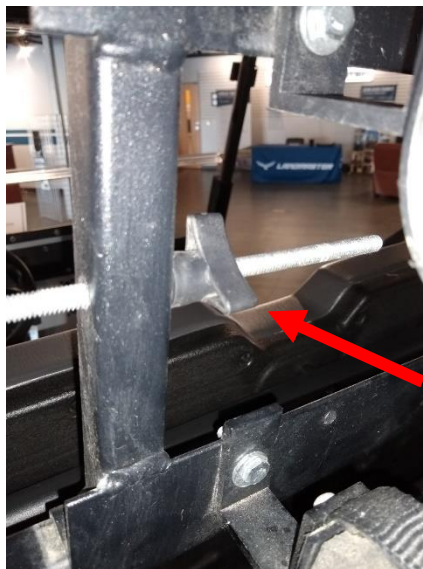
Figure 4: Tightening knob to clamp the gun rack onto the b-pillar of the vehicle.
