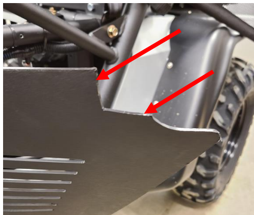
Figure 24: One inch square section of the surround cut out 19151 Installation Guide, Brake & Tail Light Package
