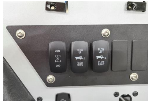
Figure 6: Switch Panel with Snow Plow Switches
