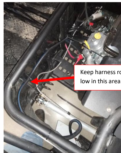
Figure 11: Bed Lift Harness Tie Wrapped in Place
