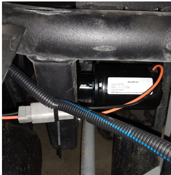
Figure 22: Mating the harness connector to the bed lift motor
