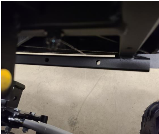
Figure 22: Location for Mounting Tail Lights
