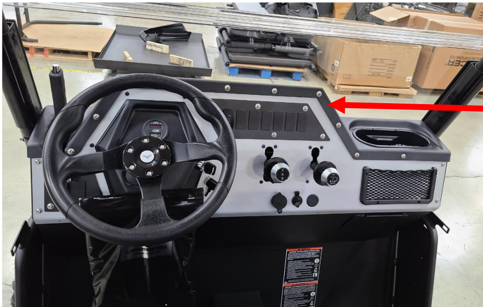
Figure 5: Removing Black Instrument Panel Cover
