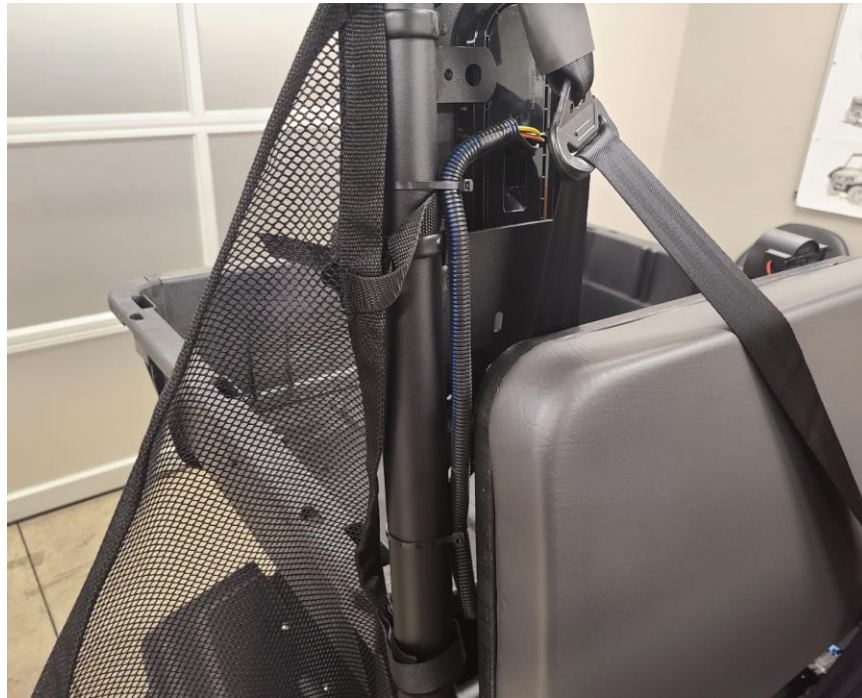
Figure 51: Route each tail light harness up to each tail light
