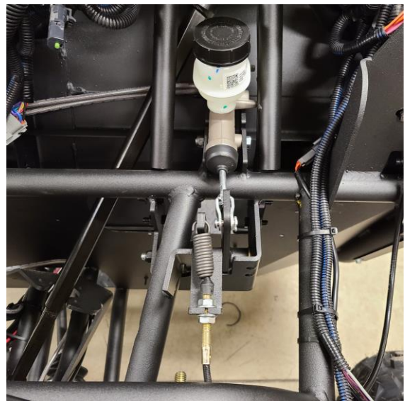
Figure 9: Brake System clam shell removed
