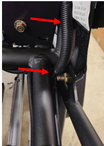
Figure 44: Route under the Side Tube
