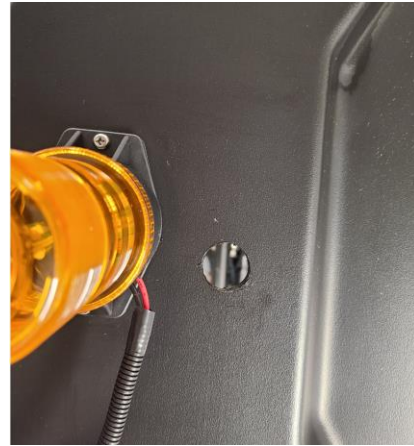
Figure 19: 1" Hole Drilled for the Harness
