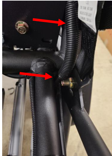
Figure 48: Route under the Side Tube
