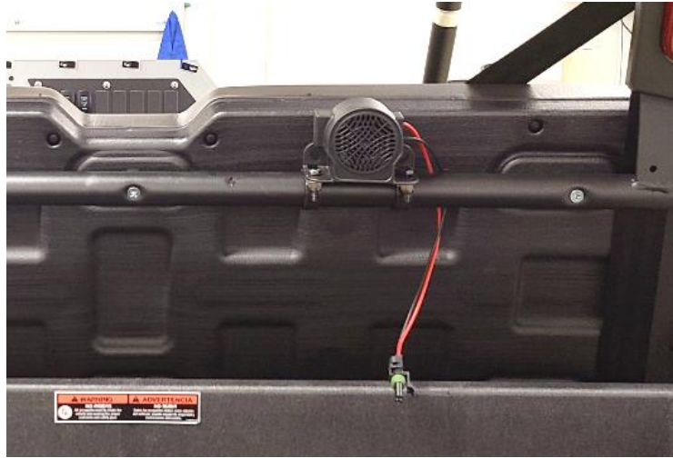
Figure 26: Backup Alarm Mounted on Upper Seat Rail
