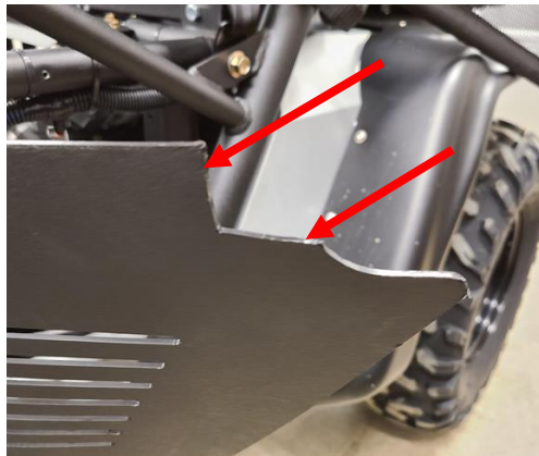
Figure 42: One inch square section of the surround cut out
