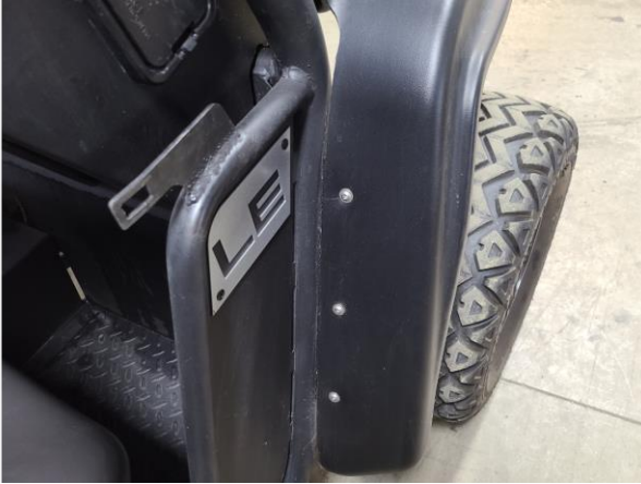
Figure 3: Removing Three Fender Fasteners
