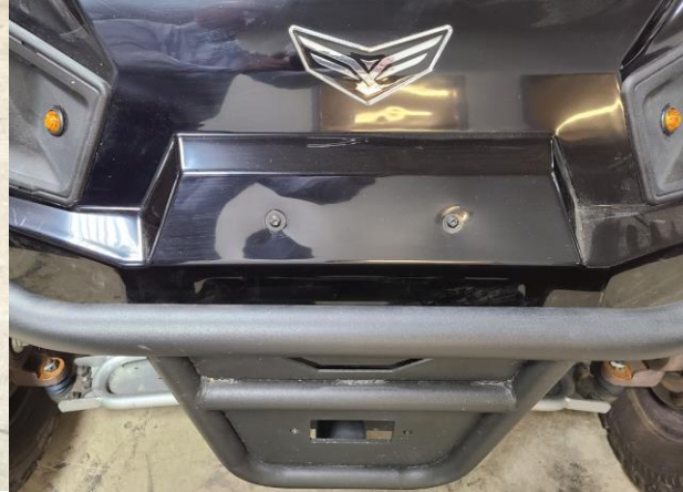
Figure 4: Removing Two Hood Fasteners
