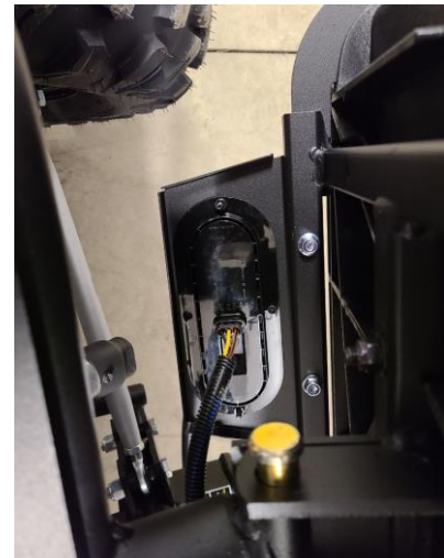
Figure 40: Tail Light Harness Connection
