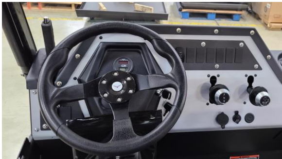
Figure 33: Seven Switch Plate in Instrument Panel
