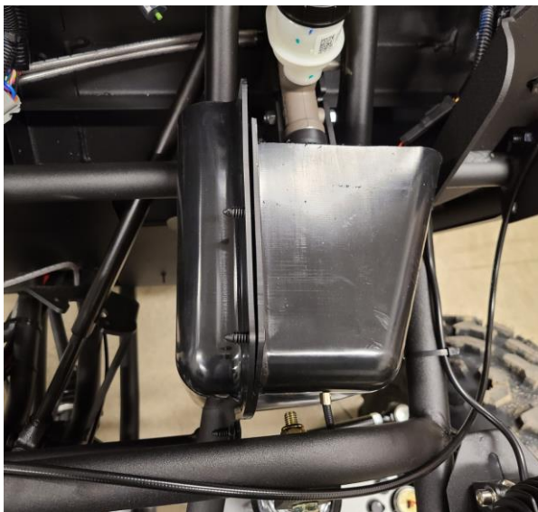
Figure 8: Brake System Clam shell housing
