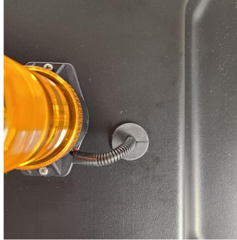
Figure 21: Grommet seated into the Roof
