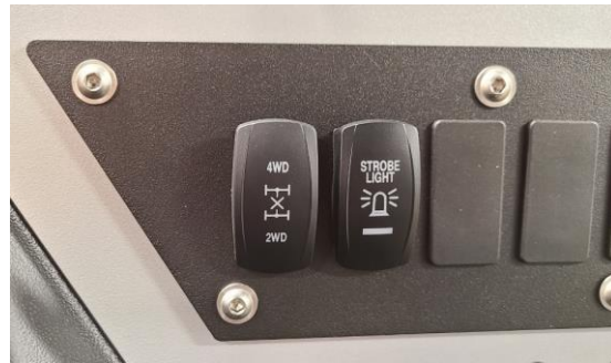
Figure 34: Seven Switch Plate with Strobe Light Switch Added
