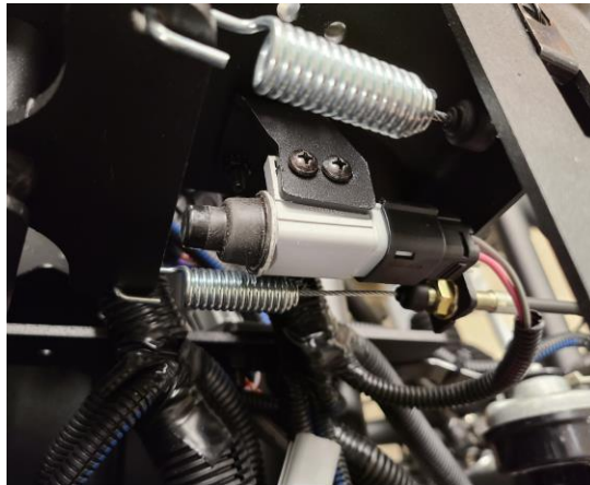
Figure 32: Backup Switch hooked up to the Harness
