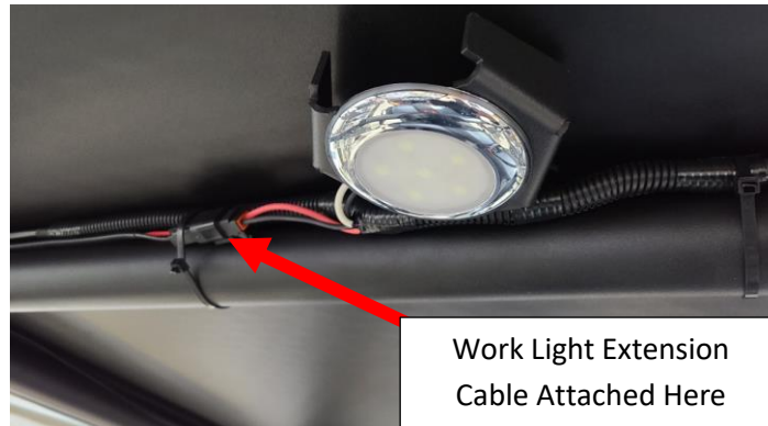
Figure 36: Work Light Extension attached to the Roof Harness
