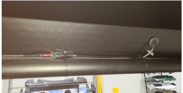
Figure 38: Extension harness attached to the Work Light
