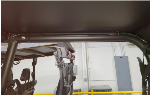
Figure 37: Extension harness routed to side rail
