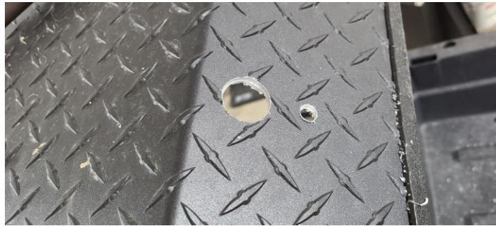
Figure 18: Holes drilled for the work lamp on the rear of the roof
