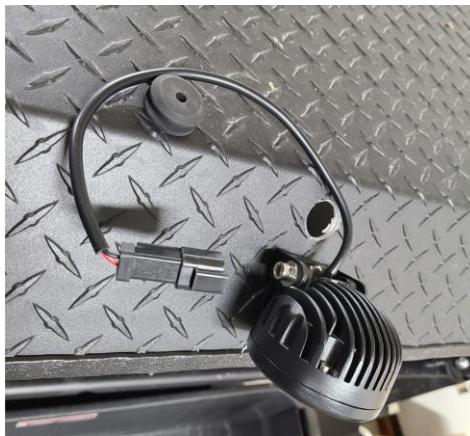
Figure 19: Work Light bolted to the roof
