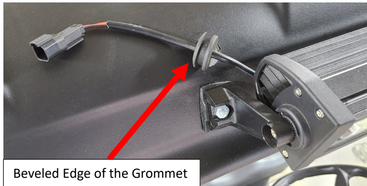
Figure 15: Grommet is attached to lamp cable
