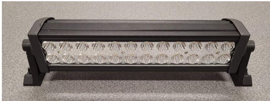
Figure 11: Lamp assembled with side brackets
