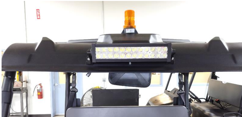
Figure 13: Flood light positioned and mounted in the Center of the Roof brow
