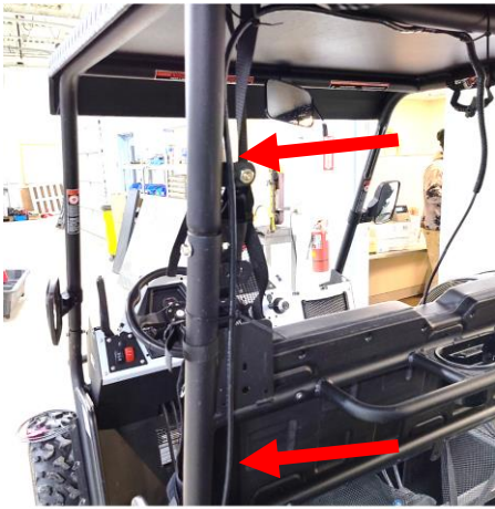
Figure 23: Cable Routed up the rear pillar Figure 24: Upper Tie Wrap Points Figure 25: Lower Tie Wrap Point
