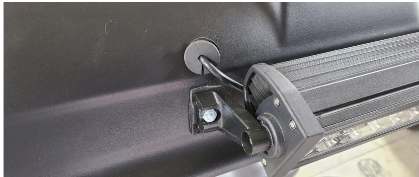
Figure 16: Grommet is started into the mounting hole
