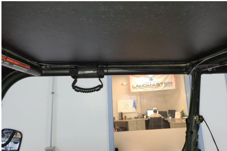
Figure 26: Flood Light harness routed along the passenger side of roof
