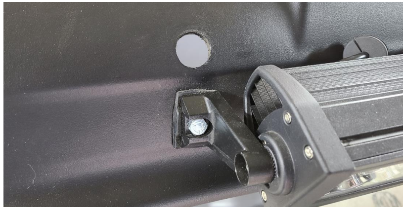
Figure 14: 1 inch hole drilled in the roof
