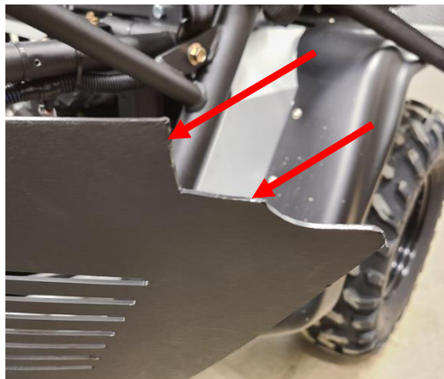
Figure 38: One inch square section of the surround cut out
