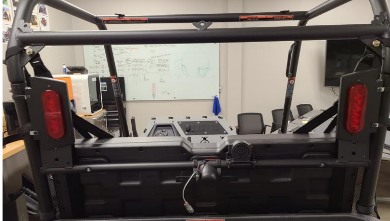
Figure 24: Tail Lights Mounted on Upper Cab Rails for Flip Seat
