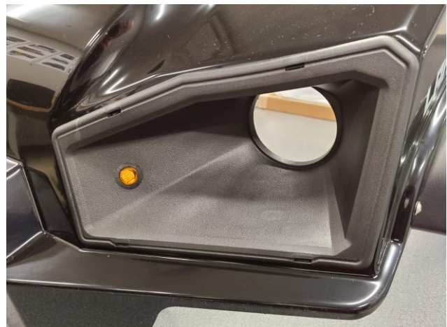
Figure 16: Front Turn Signal Lamps Installed
