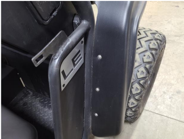
Figure 3: Removing Three Fender Fasteners
