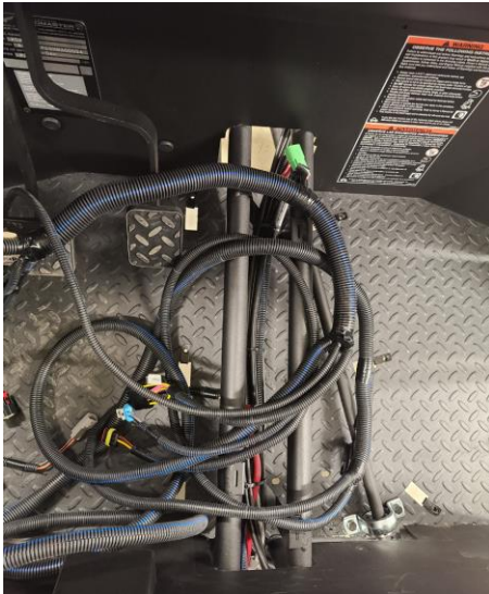
Figure 26: Harness ready to install starting at cab tunnel
