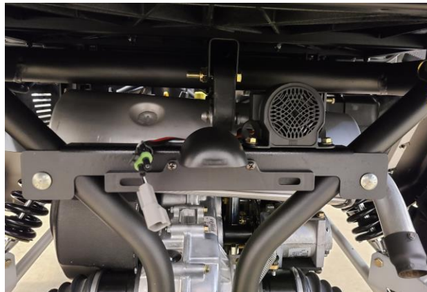
Figure 23: License Plate Light and Backup alarm Mounted to the vehicle
