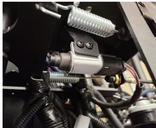
Figure 31: Backup Switch hooked up to the Harness
