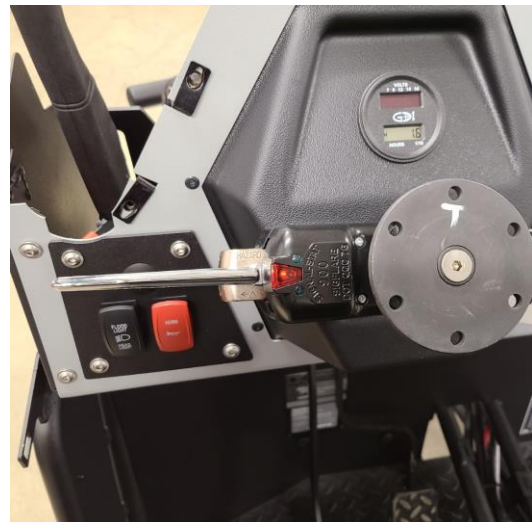
Figure 20: Hole Drilled for the Harness Connector
