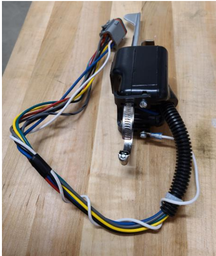
Figure 17: Turn Signal Switch with Bracket & Clamp Installed
