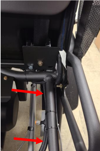
Figure 39: Routed Along Side Rail
