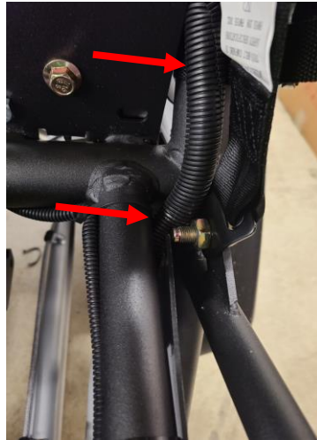
Figure 40: Route under the Side Tube
