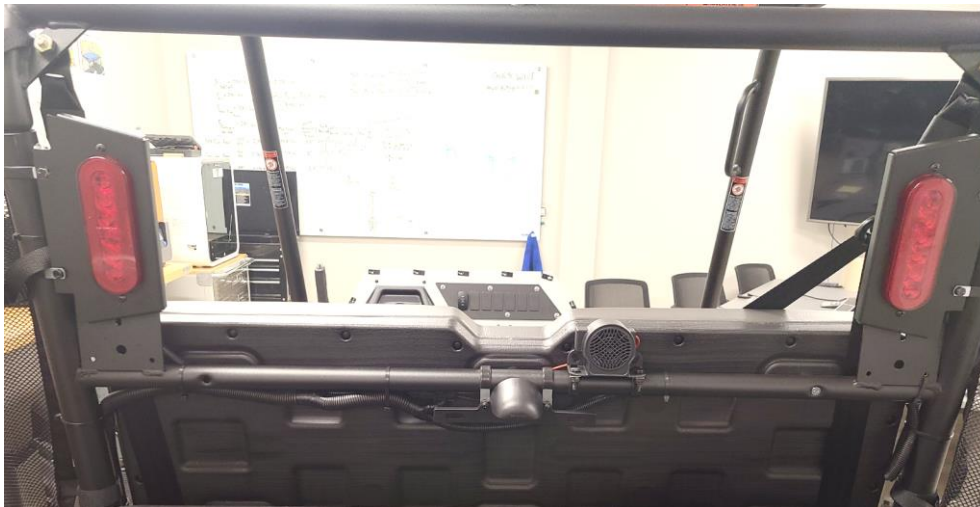
Figure 42: Harness Routed across upper seat back rail
