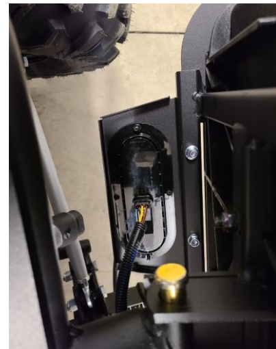
Figure 36: Tail Light Harness Connection
