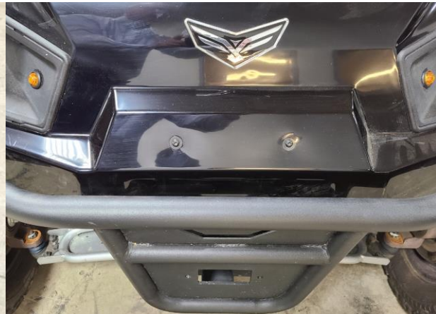
Figure 4: Removing Two Hood Fasteners
