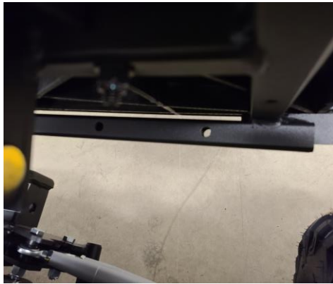
Figure 21: Location for Mounting Tail Lights
