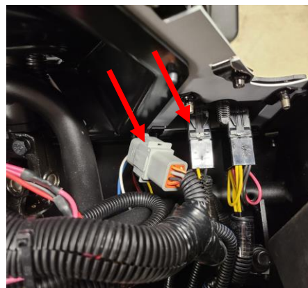
Figure 29: Horn Switch & Turn Signal Switch Hooked Up
