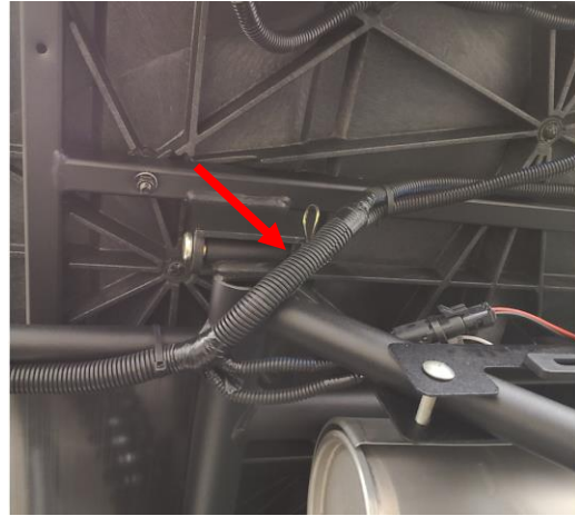
Figure 34: Harness Routed through the Pivot Point
