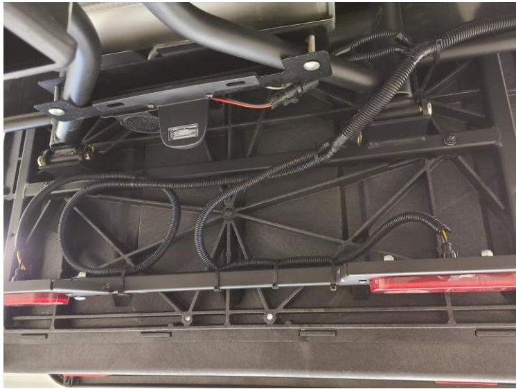
Figure 37: Tail Light Wiring Routing and Clipping on a Poly Bed
