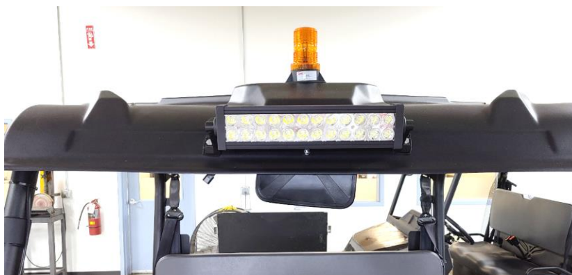
Figure 7: Flood light positioned and mounted in the Center of the Roof brow
