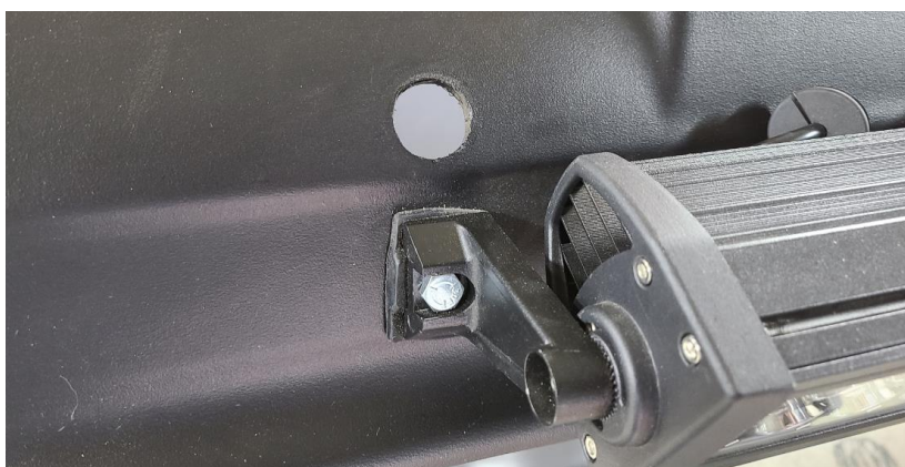
Figure 8: 1 inch hole drilled in the roof
