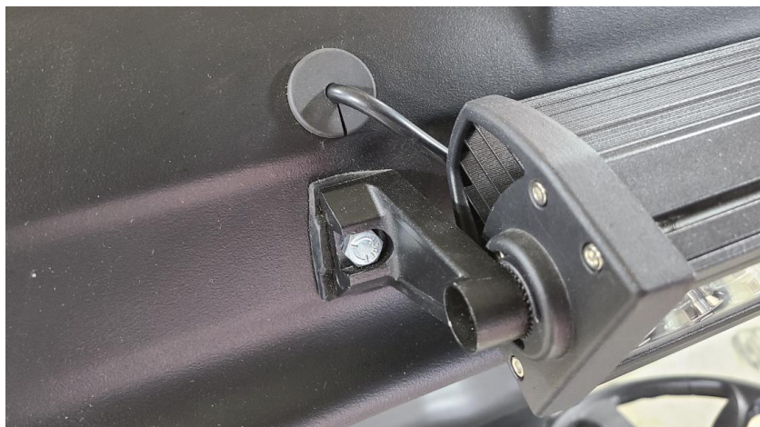
Figure 11: Grommet is fully seated in the mounting hole
