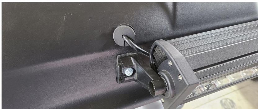
Figure 10: Grommet is started into the mounting hole
